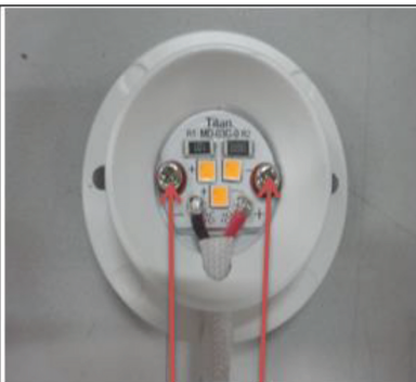
Removal of 2 screws
